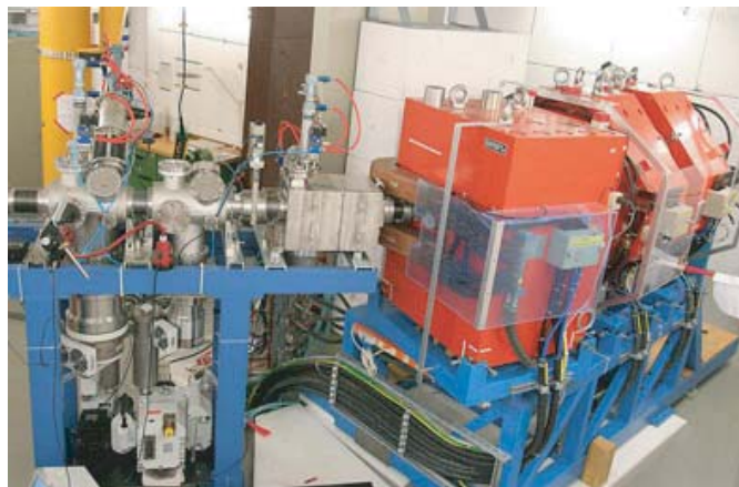
Fig. 3. (Color online) Photo of the gas-filled separator TASCA at the GSI showing (from the left) the differential pumping section which consists of two turbo pumps (below the two diagnosis chambers) and one roots pump (already installed but temporarily removed when this photo was taken), the target chamber, the dipole magnet and two quadrupole magnets.
